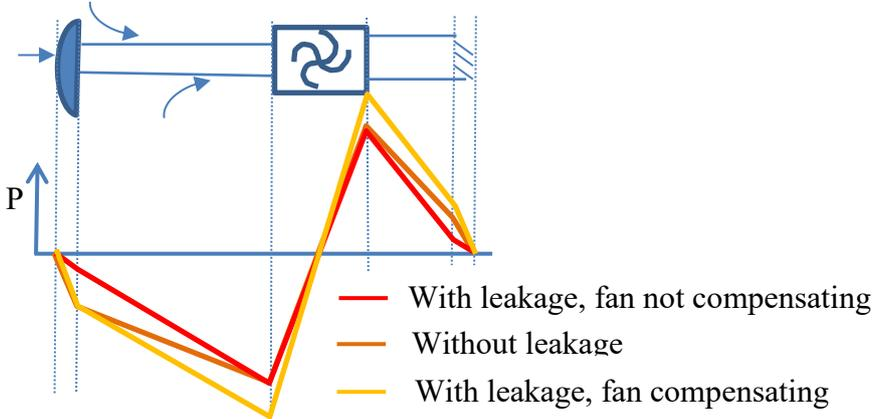
Figure 1: Pressure profile within the system with and without leakages according to the fan pressure drop. The flowrate (Q) at the Air Terminal Devices (ATD) depends upon the pressure at the ATD according to a power law.
