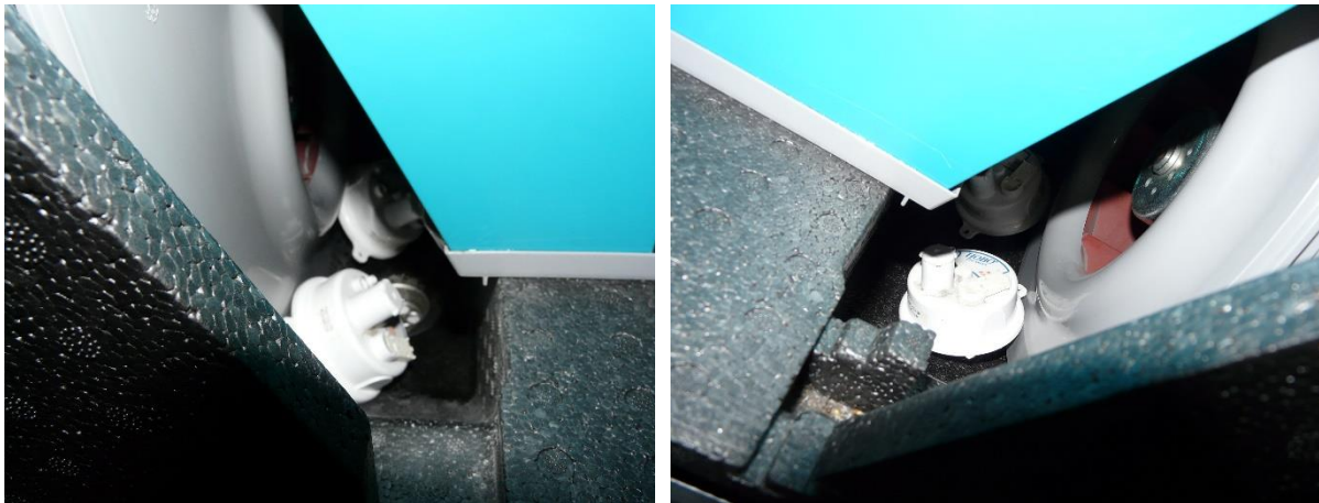
Figure 8 Positioning of the data loggers for the experiment with doubled sensors
