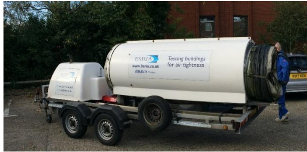
Figure 4 a petrol driven multi-gear portable trailer fan
