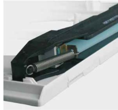
Figure 3: Close-view on the humidity sensing strip
