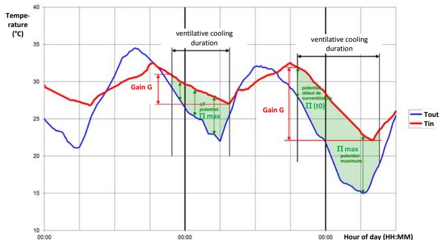
Figure 1: Thermal cooling potential  $\Pi$  and temperature Gain  $G$  based on outside and inside temperatures.
