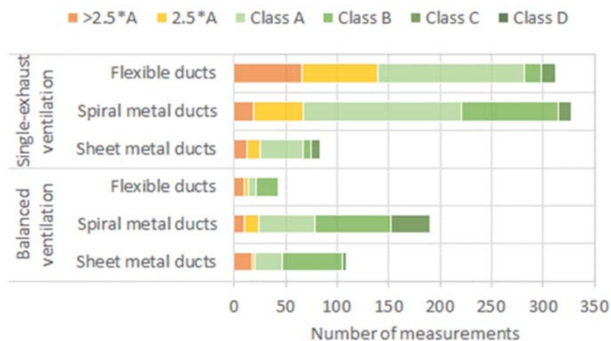
Figure 8: Distribution of ductwork airtightness measured classes depending on type of ventilation systems and implemented ducts
