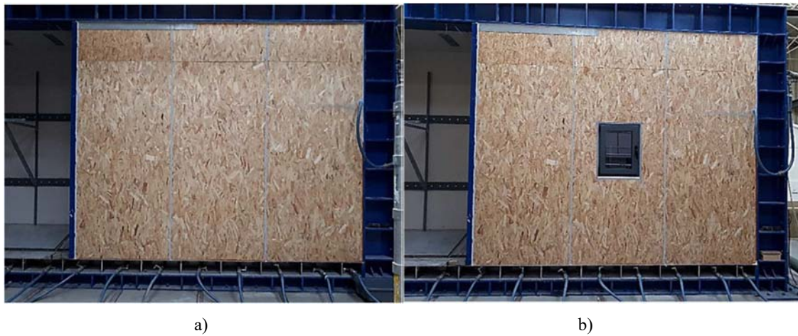
Figure 2: SIP modules tested: a) wall assembly; b) with a tilt and turn window.
