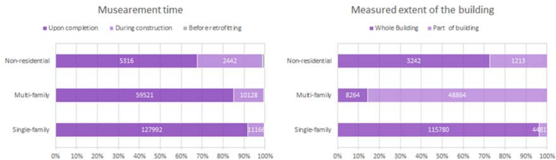
Figure 2: Number of building airtightness measurements depending on the measurement time (left) and the measured extent of building (right)
