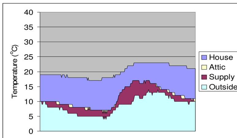
Figure 3: Supply temperature (from sunspace) pre – heats the outside air thus reducing space heating need.
