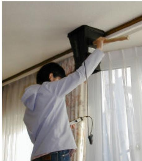
*Figure 9: Use of an airflow meter to monitor flow rates.*
