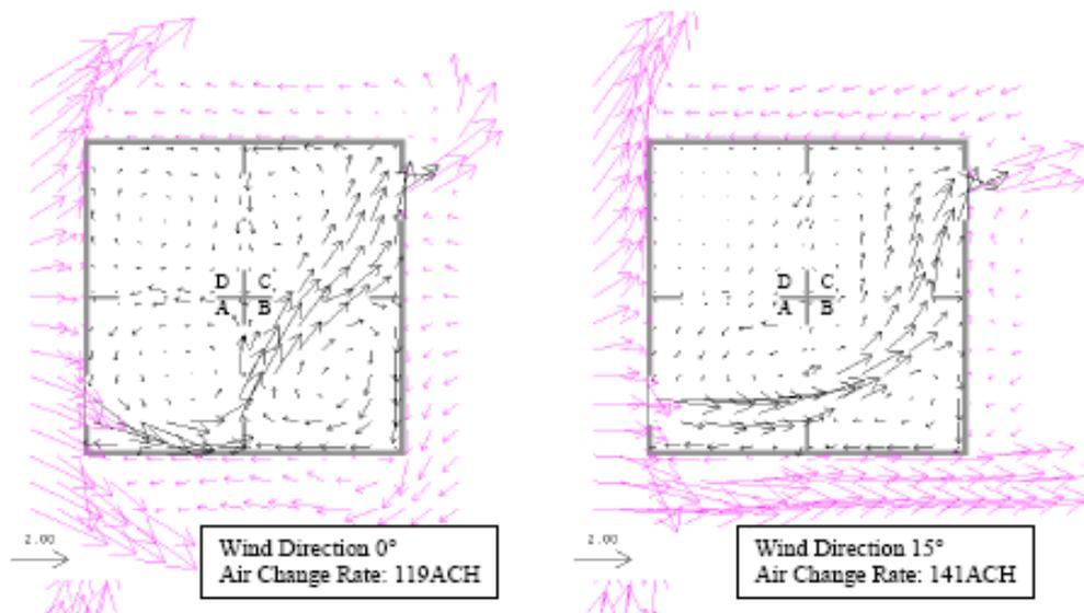
Figure 7: Examples of wind induced cross flow.
