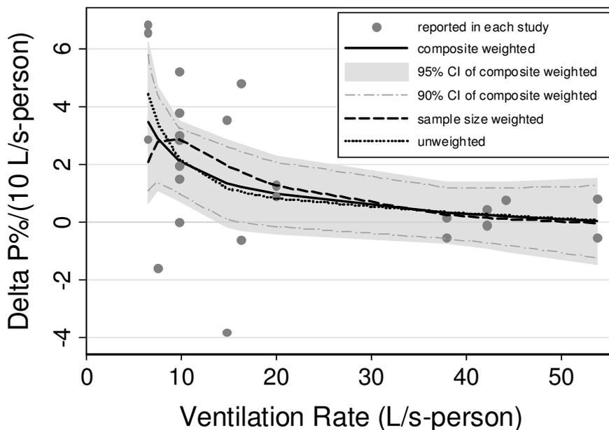
Figure 2: Increase of performance (%) vs. increase in ventilation rate of 10 L/s-person.
