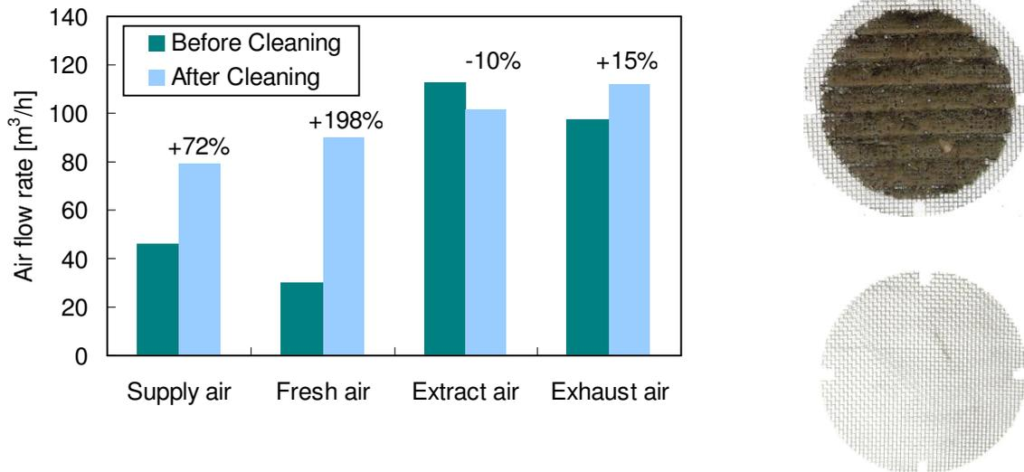
Figure 1: Cleaning has a vital impact on mechanical ventilation performance as illustrated by before and after cleaning performance.
