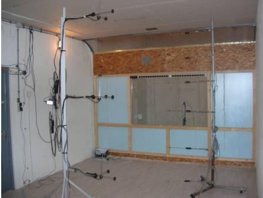
Figure 1: The climate room with test facade and measuring equipment.
