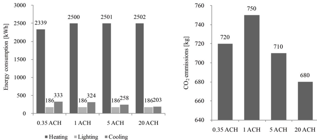
**Fig. 1** The variation in energy consumption according to changes in ventilation rates
