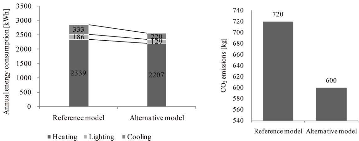
**Fig. 3** The annual energy consumption and CO<sub>2</sub> emissions of alternative model
