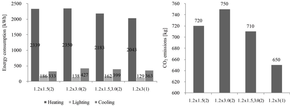
**Fig. 2** The variation in energy consumption and CO<sub>2</sub> emissions according to changes in window areas
