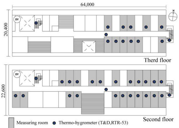
Fig. 2 Floor plan of second and third floor
