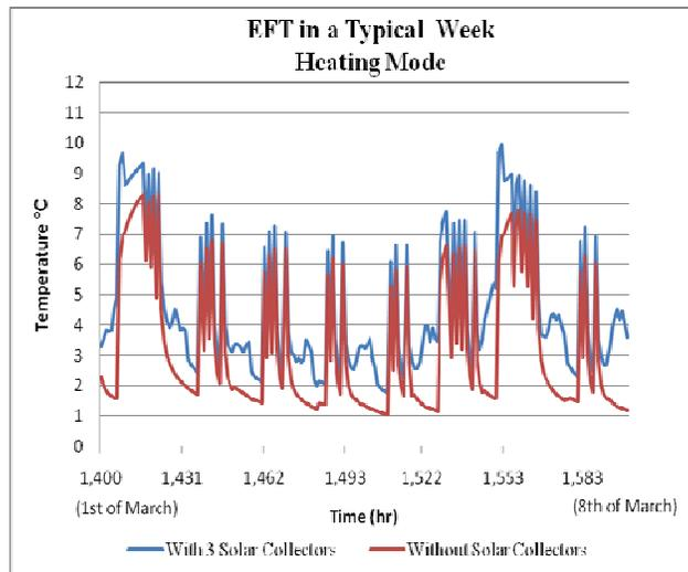
Figure 5: Heat pump EFT in a typical week of heating season
