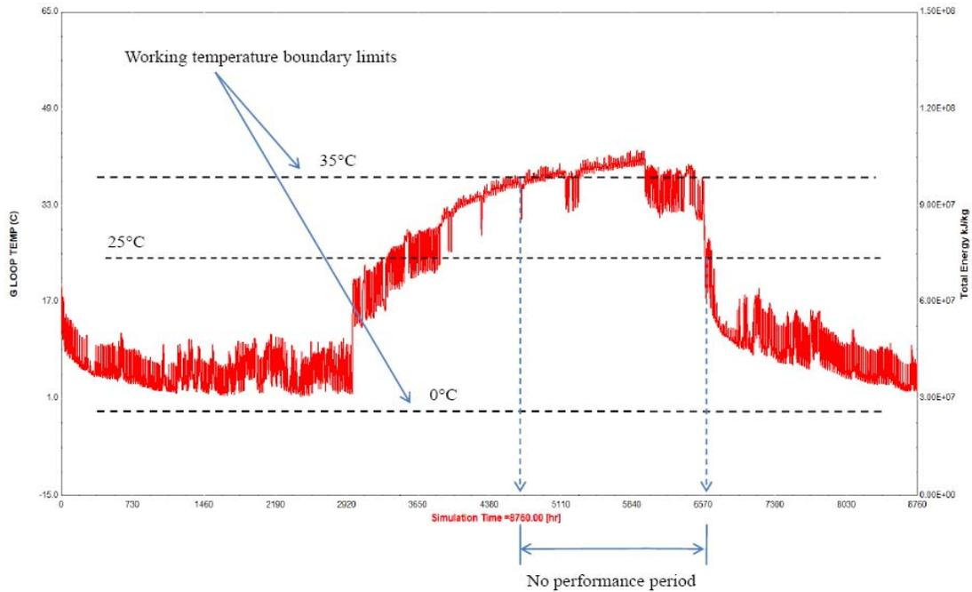
Figure 6: Existing heat pump EFT limits (System with 3 solar panels)
