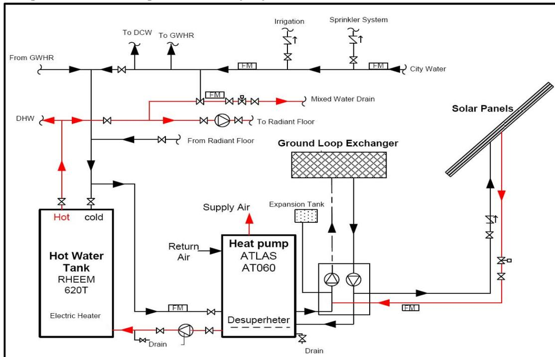
Figure 1: Schematic diagram of SAGSHP system configuration
