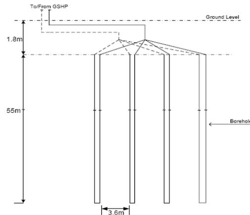
Figure 2: Ground loop borehole layout
