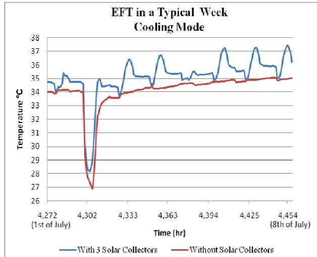
Figure 4: Heat pump EFT in a typical week of cooling season
