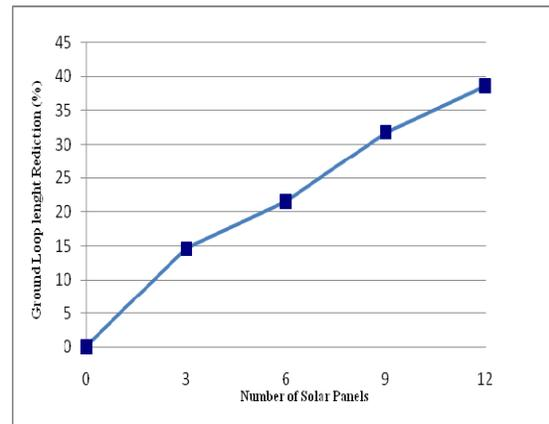
Figure 3: Ground loop length reduction percentage versus number of solar panels
