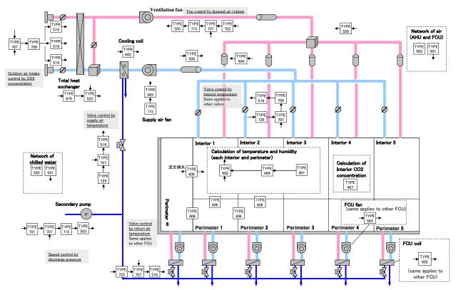
Figure 5 System configuration of HVAC systems on the model floor
