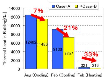
Figure 9 Energy change of loads by changing air conditioner preset temperatures
