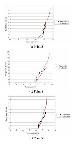
Figure 12 Compared CFD results with measurement results of vertical air temperature profiles
