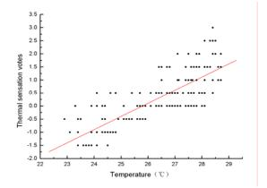
Figure 11 Calculation of thermal neutral temperatures in summer conditions
