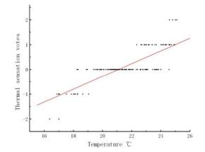
Figure 10 Calculation of thermal neutral temperatures in winter conditions
