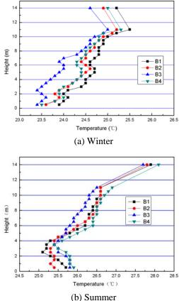
Figure 9 Vertical temperature of measurement Point 2, 5 and 7 in Check-in Hall
