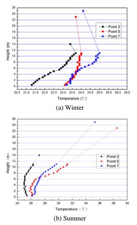
Figure 7 Vertical temperature of measurement Point 2, 5 and 7 in Check-in Hall
