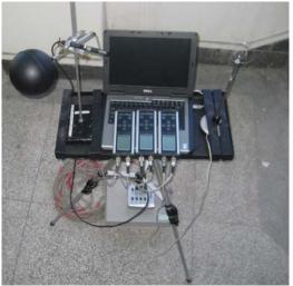
Figure 5 Thermal comfort meter
