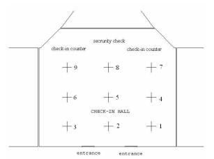
Figure 4 Distributions of the site-measurements of Check-in Hall
