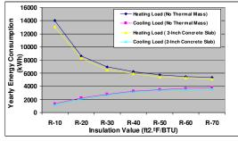
Figure 8: Comparison of the impact on the heating and cooling loads as insulation levels are varied when thermal mass is used versus no thermal mass
