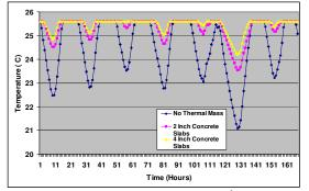
Figure 6: Temperature profile of the 3<sup>rd</sup> floor of the Net Zero Energy house during a typical summer week with varying thermal mass
