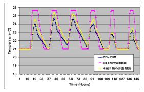
Figure 7: Temperature profile comparing the thermal mass effect of 20% Micronal PCM and 4-Inch Concrete Slab for the 3<sup>rd</sup> floor of the Net Zero Energy house during a typical winter week.
