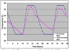
Figure 10: Temperature profile of the 3rd Floor of the house for a 48-hour duration for the winter season,, comparing the impact of using a 4-inch thick concrete slab
