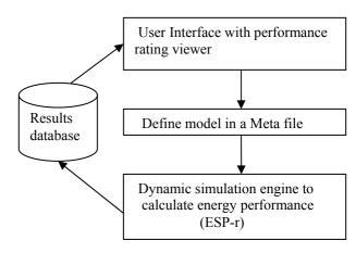
Figure 2 Architecture of EDEM-SAMSUNG
