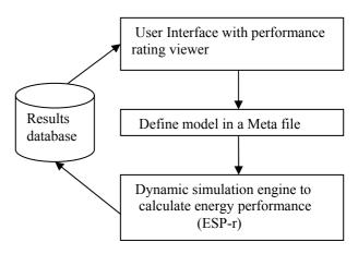
Figure 2 Architecture of EDEM-SAMSUNG
