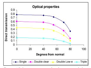
Figure 4 Solar transmittance for glazing provided in EDEM-Samsung
