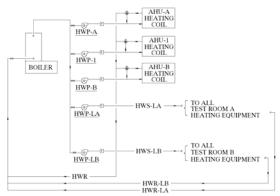
Figure 4: Simplified heating water piping schematic
