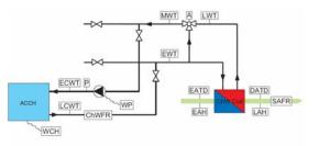
Figure 1: Scheme of the chilled water system with measuring points
