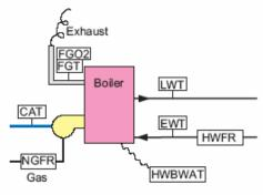
Figure 5: Scheme of the condensing boiler with measuring points
