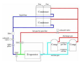
Figure 3: Air-cooled chiller refrigeration circuit
