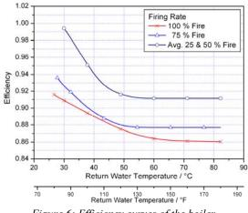
*Figure 6: Efficiency curves of the boiler*
