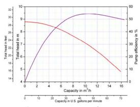
Figure 8: Heating water pump performance curve extract
