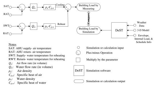
Figure 2 Block diagram of model calibration
