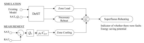
Figure 4 Block diagram of fault detection
