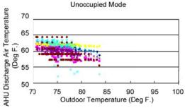
Figure 7 Optimal AHU supply-air temperature by simulating
