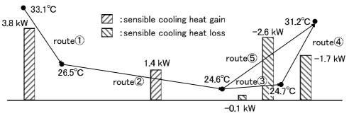
Figure 10 Air temperature at each measurement point and sensible cooling heat gain/loss in air introduce route
