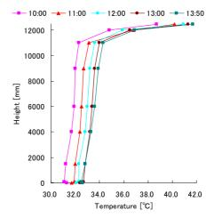
Figure 5 Indoor vertical air temperature distribution on Aug.11 (without natural ventilation)
