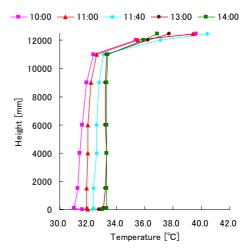
Figure 6 Indoor vertical air temperature distribution on Aug.14 (natural ventilation)
