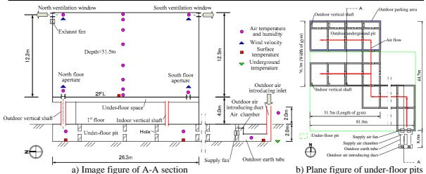
Figure 2 Imagine figures of the coupled earth tube and natural ventilation system and measurement points
