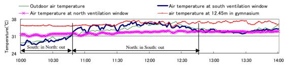
Figure 7 Outdoor air temperature, air temperature at south/north ventilation window and at 12.45m in gymnasium (Aug.14, natural ventilation)
