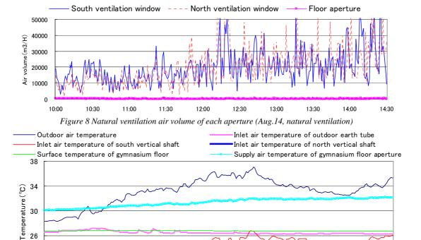
Figure 9 Outdoor air temperature, air temperature at each measurement point in air introduce route and floor surface temperature of gymnasium (Aug. 14, natural ventilation)
