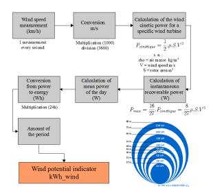
Figure 13. Wind potential estimation.
