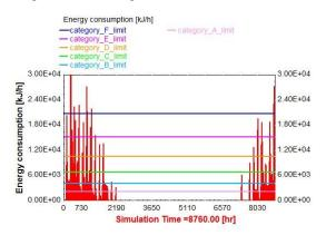
Figure 2. Energy consumption compared to energy performance categories.
