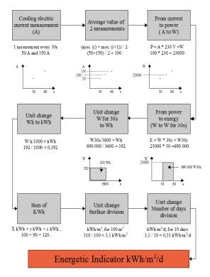
Figure 9. Air-conditioning consumption algorithm.
