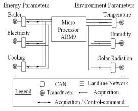
Figure 5. BEMS communication scheme.
