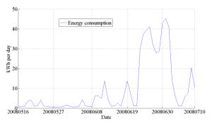
Figure 10. Daily energy consumption of the airconditioning system.
