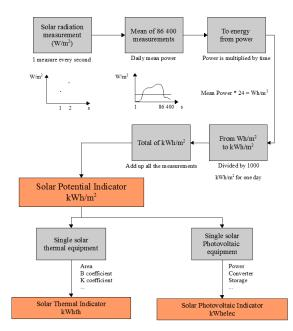
Figure 12. Solar potential estimation.
