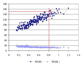
Figure 6 Infiltration rate compared to weighted over and under heating hours
