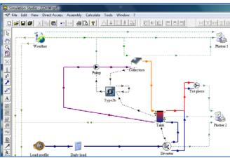
Figure 1 Example Project in Simulation Studio
