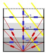
Figure 4 Radiative zone with 3 air nodes
