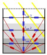
Figure 4 Radiative zone with 3 air nodes
