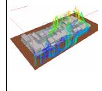
Figure 7 Streamlines for houses facing prevailing SE winds.
