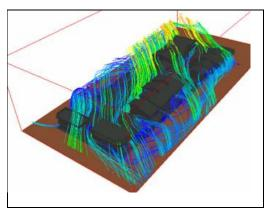
Figure 9 Streamlines originated at east and west façades.
