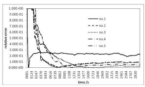
Fig.7 Relative error of CO<sub>2</sub> concentrations between test and calculation
