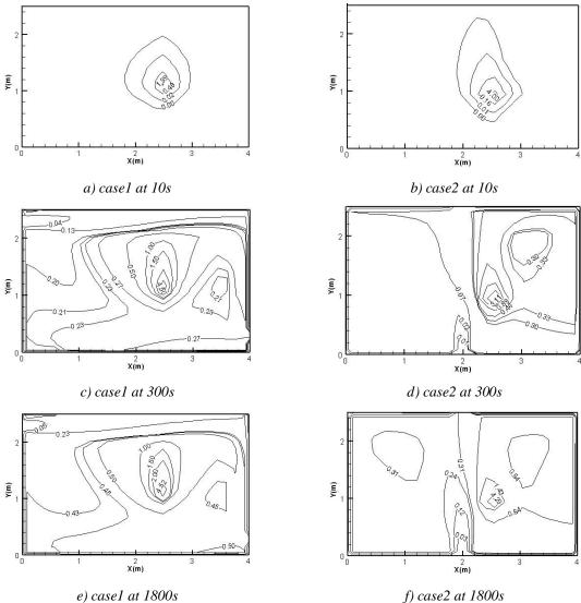
Fig. 5. Contaminant distributions of SCHEME2 (mg/m3, section Z=1.5m)
