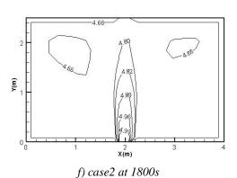
CHEME1 (mg/m3, section Z=1.5m) approached uniform with time. That means for these two cases, the influence of airflow is small.
