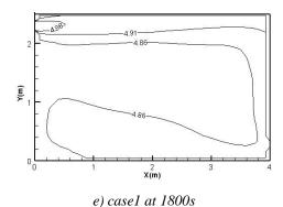
Fig. 4. Contaminant distributions of SCHEME1 (mg/m3, section Z=1.5m)
