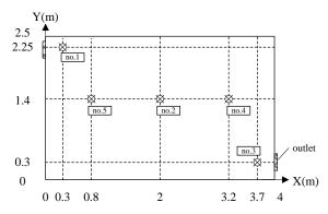
Fig. 6. Configuration of the test chamber
