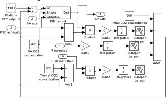
Figure 4 CO<sub>2</sub> control sub-model
