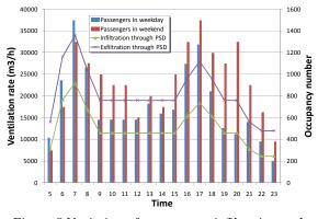
Figure 8 Variation of passengers, infiltration and exfiltration rate through PSDs
