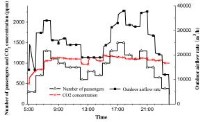
Figure 9 The variation of number of passengers, CO<sub>2</sub> concentration and outdoor airflow rate
