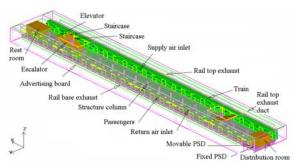
Figure 2 Three-dimensional model of subway island platform
