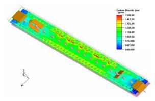
Figure 3  $CO_2$  concentration distribution at the height of 1.65m above the platform
