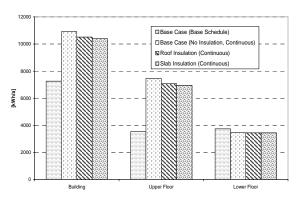
Figure 14 Comparison of annual cooling energy as the effect of operational time of the cooling device
