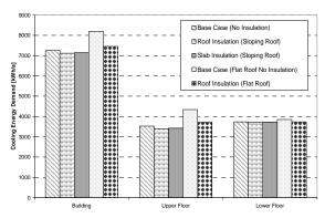
Figure 15 Comparison of annual cooling energy between sloping roof and flat roof
