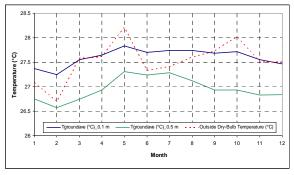
Figure 4. Ground Temperature Profile
