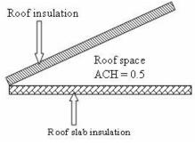
Figure 5 Roof insulation installation.
