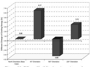
Figure 10 Effect of building's orientation to the cooling energy demand.
