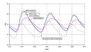
Figure 6 Temperature profile inside roof space
