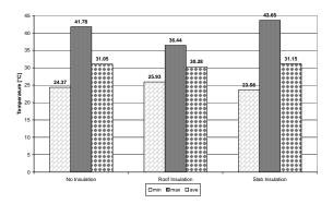
Figure 9 Comparison of minimum, maximum and average temperature inside roof space
