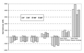
Figure 11 Comparison of heat transfer through building envelopes for different building orientation
