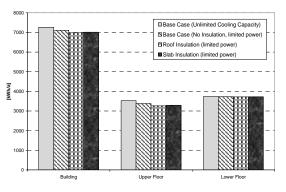
Figure 13 Comparison of annual cooling energy as the effect of limited power of the cooling device.
