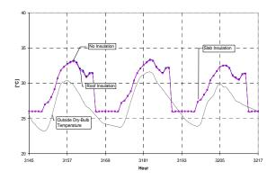
Figure 7 Temperature profile of upper floor
