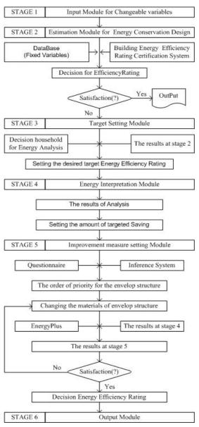
Figure 2 Flow chart of the support system
