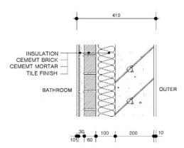
Figure 1 Typical structure of the outer wall
