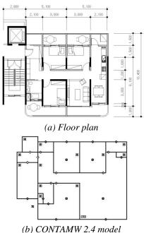
Figure 2 Floor plan and CONTAMW 2.4 model
