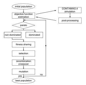
Figure 2 Integration of the GA, Pareto optimality with CONTAMW 2.4 simulation
