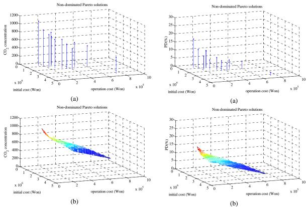
Figure 4 18 Pareto optimal solutions #1 (XYZ: investment cost, operation cost, CO<sub>2</sub> concentration)
