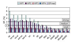
Figure 7 Daylight Factor in the four work planes
