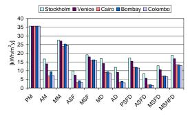
Figure 8 Energy requirement for artificial lighting, for the five investigated places, considering users' behaviour and different control strategies
