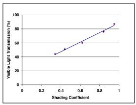
Figure 6: Relationship between shading coefficient and visible light transmittance for the glazing selected.
