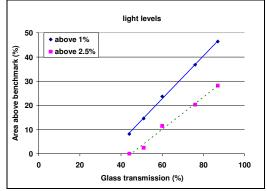
Figure 10: Comparison of area above the 1% and 2.5% daylight factor threshold and the glazing transmission.
