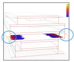
Figure 7: Section with light shelves on modelled floor.
