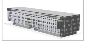
Figure 4: Western Façade showing vertical shading fins
