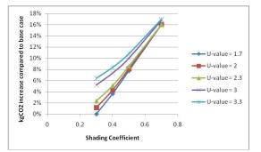
Figure 8: Comparison of emissions with base case depending on variations of shading coefficient and U-Value of the glazing with vertical fins.
