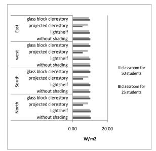
Figure 8 Hourly heat flows through the building fabrics
