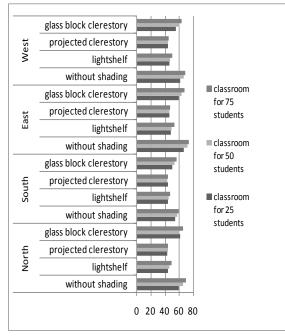
Figure 2 Hourly Thermal Transfer Value (W/m<sup>2</sup>) of Window with 34-39% WWR
