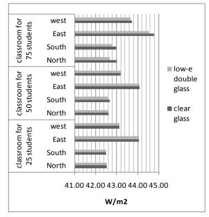
Figure 9 Comparison of Hourly Thermal Transfer Value (W/m<sup>2</sup>) between projected clerestory with single glazing and with double glazing low-e
