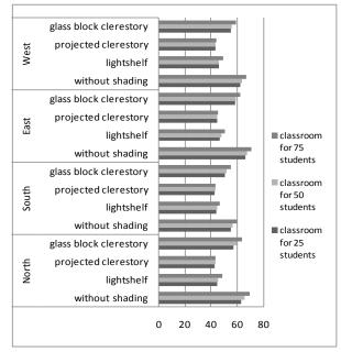
Figure 3 Hourly Thermal Transfer Value (W/m<sup>2</sup>) of Window with 20% WWR
