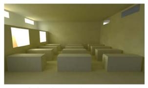
Figure 6 Three dimensional picture of a classroom for 25 students with projected clerestory is resulted by Radiance (link to Ecotect) simulation.
