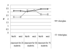
Figure 10 Comparison of average daylight factor between projected clerestory window with clear glass and with tinted glass
