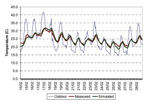
Figure 6 Two weeks summer comparison of simulated and measured temperatures in the living room of house 2
