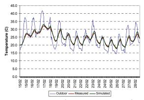
Figure 7 Two weeks summer comparison of simulated and measured temperatures in the living room of house 3
