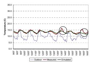
Figure 4 One-week winter comparison of simulated and measured temperatures in the living room of house 1 indicating the use of a space heater in the actual house (in circles)
