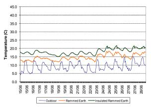
Figure 8 Two weeks of predicted temperatures in winter if house 3 used only rammed earth walls
