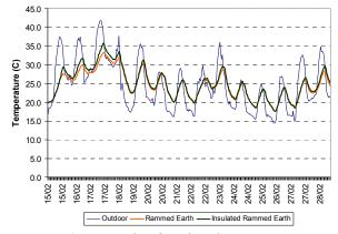
Figure 9 Two weeks of predicted temperatures in summer if house 3 used only rammed earth walls
