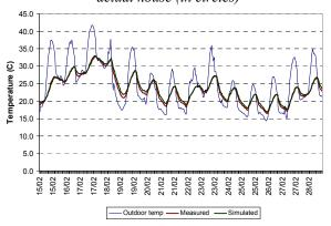
Figure 5 Two weeks summer comparison of simulated and measured temperatures in the living room of house 1
