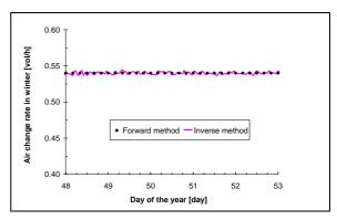
Figure 7: Air change rate with forward and inverse methods during winter
