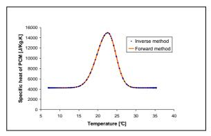
Figure 4: Comparison of the theoretical heat capacity and heat capacity evaluated by the inverse method
