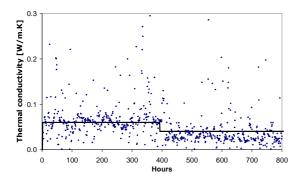
Figure 11: Estimated value of the multilayered wall thermal conductivity
