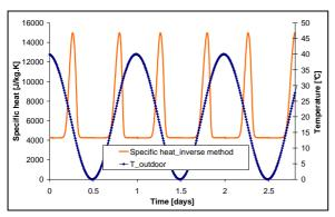
Figure 5: Heat capacity in a node of PCM
