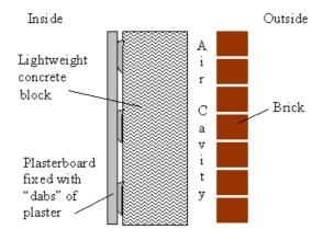
Figure 10: Section of the monitored wall
