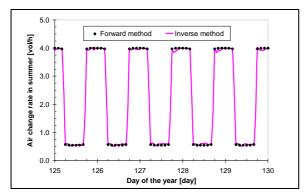
Figure 8: Air change rate with forward and inverse methods in summer (with over-ventilation)
