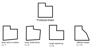
Figure 6. Differences in Difference factor  $\boldsymbol{D}$  between similar plan forms.
