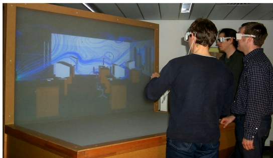
Figure 14: Computational steering means interacting with an ongoing (e.g. CFD) simulation, for example using a holobench with space pointing device (picture courtesy of TUM and LRZ, Germany)
