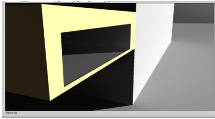
Figure 6 Radiance render of a COMFEN floor to ceiling glass scenario for an office with allowance for a plenum
