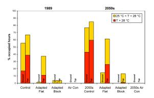
Figure 8 Living rooms in flats: Percentage of occupied hours exceeding CIBSE comfort temperature, 25 °C is shown by total size of bars. Hours during which the CIBSE overheating temperature, 28 °C, is exceeded, are shown in red.
