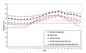
Figure 5 Operative Temperature profiles for the hottest day for house living room
