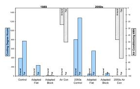
Figure 9 Flat Living Room: July CDH. The right hand axis shows air conditioning power consumption (in kWh) required to control overheating in the air-conditioned cases.
