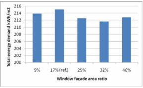
Figure 12 The building's total energy demand (kWh/m²) with respect to the 'window façade area ratio'.
