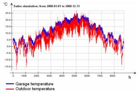
Figure 5 Air temperatures in the parking space in comparison with the outdoor temperatures.
