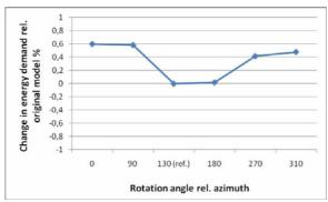
Figure 10 Percentage of change in energy demand dependent on the building's orientation.
