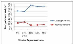
Figure 14 Energy demands (kWh/m²) for cooling and heating for different window façade area ratios.
