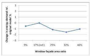
Figure 13 Percentage of change in energy demand dependent on the 'window façade area ratio'.
