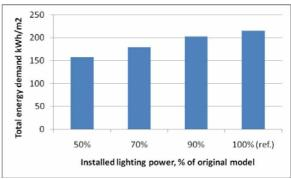
Figure 15 The building's total energy demand (kWh/m<sup>2</sup>) with respect to installed lighting power.
