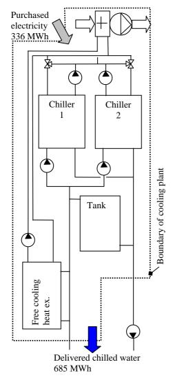
Figure 8 Principle scheme of the cooling plant in the model. The definition of COP<sub>system</sub> in this paper is defined as delivered chilled water divided by purchased electricity to the cooling plant.
