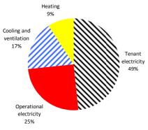
Figure 2 Distribution of electricity use by percentage in the reference building divided between: electricity use in shops, electricity for building operation, space cooling and ventilation, and space heating.
