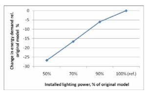
Figure 16 Percentage of change in energy demand dependent on the installed lighting power.
