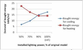
Figure 18 Demand of bought energy (kWh/m²) for heating and cooling depending on installed lighting power in the model's shop zones.
