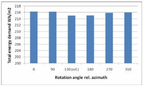
Figure 9 The building's total energy demand  $(kWh/m^2)$  with respect to building orientation.
