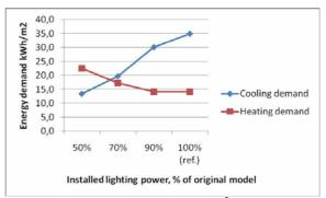
Figure 17 Energy demands (kWh/m<sup>2</sup>) for cooling and heating for different installed lighting powers.
