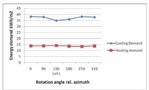
Figure 11 Energy demands (kWh/m<sup>2</sup>) for cooling and heating for different building orientations.
