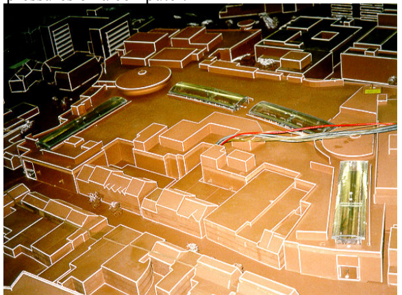
Figure 4 Wind tunnel model showing pressure tubes
