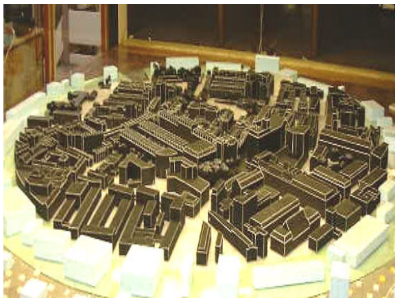
Figure 2 Wind tunnel model with surrounding buildings
