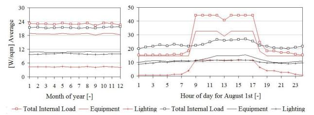
Figure 8 Updated model (black), using actual measured data, vs. initial model (red) energy use per floor area.
