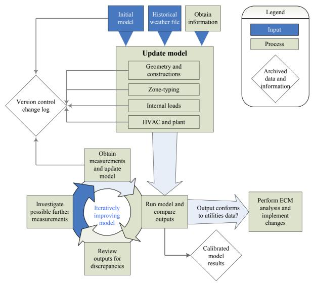
Figure 1 Calibration methodology
