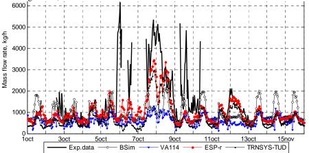
Figure 10. Hourly averaged mass flow rate in the DSF cavity, measured with the tracer gas method. DSF200\_e.
