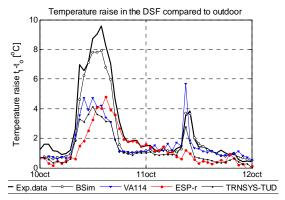
Figure 8. Temperature rise in the DSF cavity compared to the outdoor air temperature. DSF\_200e. Cooling/heating power in exp.room
