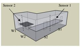
Figure 8 Case Study #3 sensor plane locations and facade sections
