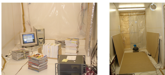
Figure 4 Test setup in the climatic chamber in the VLIET-test building
