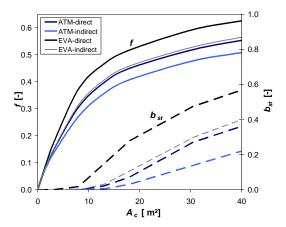
Figure 8 Solar combisystem performance characteristics for investigated variants
