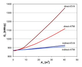
Figure 10 Space cooling demand increase induced by solar collector integration into façade
