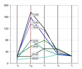
Figure 2 Temperature profiles in façade with directly integrated atmospheric flat-plate collector during summer day
