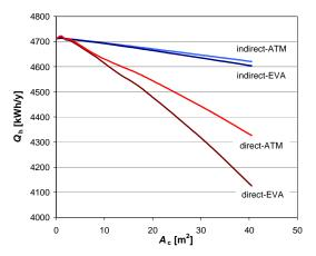
Figure 9 Space heating demand decrease induced by solar collector integration into façade
