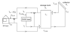
Figure 7 Solar combisystem model layout
