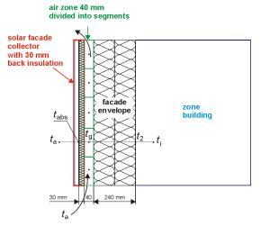
Figure 5 Indirect integration with ventilated air gap.
