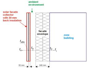
Figure 3 Indirect integration of solar collector considered as a separate installation
