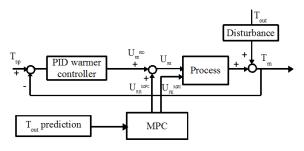
Figure 5. MPC control framework.
