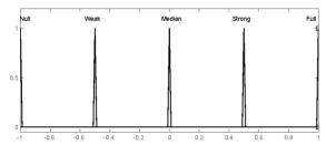
Figure 10. Fuzzification of normalized  $U_{RE}^{FLC}$ .
