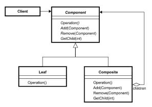
Fig. 9 UML class diagrams of Composite pattern
