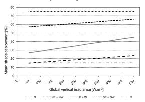
Figure 14 Dependency model of shades deployment level (in %) as a function of façade orientation (S: South, NE: North-East, NW: North-West, E: East, W: West, SE: South-East, SW: South-West, S: South) and the incident global (vertical) irradiance on the façade
