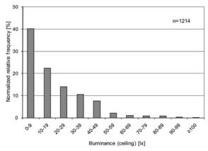
Figure 5 Normalized relative frequency of 'switch on' actions (0-500 lx) in UT as a function of ceiling illuminance (6:00 to 18:00, all shades open)
