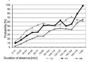
Figure 7 Probability of switching the lights off as a function of the duration of absence (in minutes) from the offices in VC, FH, and HB
