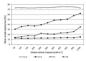
Figure 8 Mean shade deployment degree (VC-S, VC-S, FH, and HB) as a function of global vertical irradiance incident on the façade
