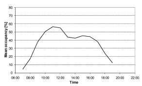
Figure 11 Mean occupancy input model for building performance simulation applications
