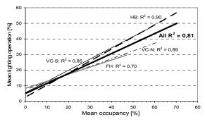
Figure 3 Lighting operation (in % of maximum installed load) in relation to mean occupancy for all time intervals of the working hours during the observation period in VC-N, VC-S, FH, and HB offices (shown is also the regression line for all observations)
