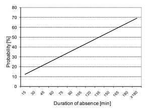
Figure 13 Light switch off probability model based on duration of absence from the workstation
