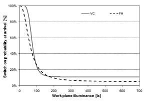
Figure 4 Probability of switching the lights on upon arrival in the office in VC and FH as a function of the prevailing task illuminance level
