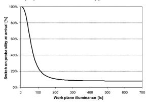
Figure 12 Light switch on probability model based on task illuminance level immediately prior to the onset of occupancy
