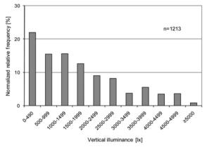
Figure 6 Normalized relative frequency of 'switch on' actions (0-500 lx) as a function of vertical illuminance (intervals between 6:00 and 18:00 with shades open)
