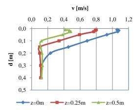
Figure 4 Measured velocity profiles
