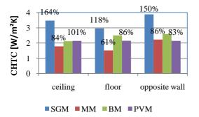
Figure 4 CHTC at three enclosure walls for different diffuser models
