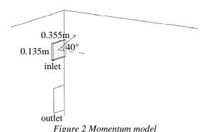
The momentum force of the added source is determined by the difference between the effective momentum and the momentum originating from the simplified opening. The momentum force F is described by (9). In this equation v represents the velocity magnitude at the exit of the nozzle opening in case of the effective momentum, respectively the simplified gross outflow surface. In the former case, A corresponds with the effective area, while in the latter, A stands for the gross area.
