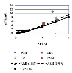
Figure 6 Convective heat flux at the opposite wall: empirical correlations and simulated values
