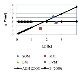
Figure 5 Convective heat flux at the ceiling: empirical correlations and simulated values
